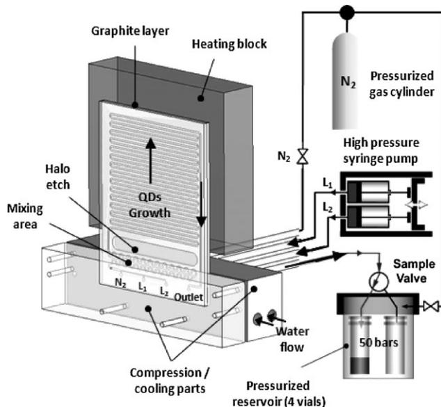
**Figure 1.** Experimental set-up including a high-pressure high-temperature microreactor, a compression-cooling aluminum part, a high-pressure syringe pump, a 5-way high-pressure valve, and a high-pressure reservoir containing 4 vials.
