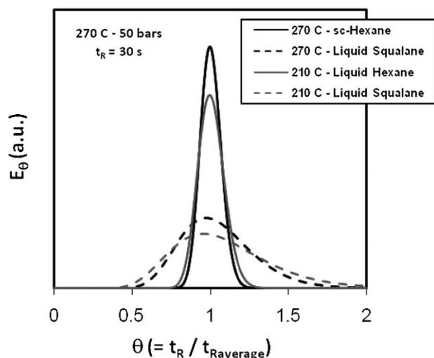
**Figure 4.** RTD curve calculated using a Taylor dispersion model for hexane and squalane at 210 °C, 5 MPa and 270 °C in a 400  $\mu\text{m}$   $\times$  250  $\mu\text{m}$   $\times$  1 m microchannel for a residence time of 30 s.
