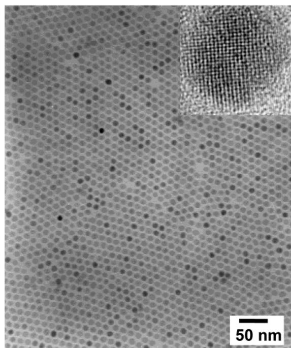
**Figure 2.** TEM image of a two-dimensional hexagonally close-packed assembly and high-resolution TEM image (inset) of 9 nm cobalt ferrite nanocrystals. Low-resolution TEM images were obtained on a JEOL EM-2000 EX II microscope, and HRTEM images were taken on a JEOL JEM-3000F microscope.
