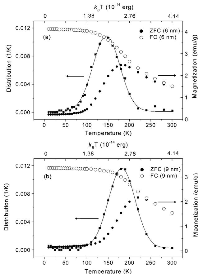
**Figure 4.** Zero-field-cooled (●) and field-cooled (○) magnetization data measured in an applied field of 100 Oe, and energy barrier distributions of magnetic anisotropy (■) of (a) 6 nm and (b) 9 nm cobalt ferrite nanocrystals. The energy barrier distributions of magnetic anisotropy are fitted well using Gaussian functions (solid lines).
