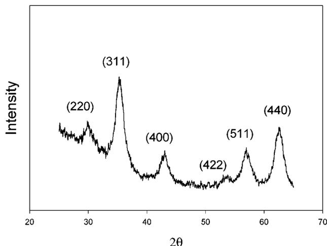
**Figure 3.** X-ray diffraction pattern of 6 nm cobalt ferrite nanocrystals obtained with a Rigaku D/Max-3C diffractometer equipped with a rotating anode and a Cu K $\alpha$  radiation source ( $\lambda = 0.154\ 056$  nm).
